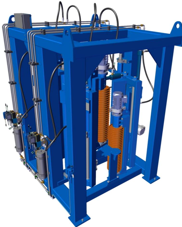
**LOG TURNER VLT-1200** consists of double pairs of vertical serrated rolls with servo-hydraulic centering and separate drives. The four rollers are movable vertically, i.e. up and down via a guide system.
