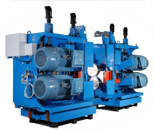
QSS-420/S6 is a double-arbor circular saw that can be placed as a rotary gang saw, close coupled with a chipper canter or as stand-alone with a centering feed-work.
