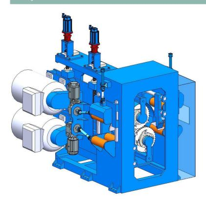
DSS-300F is a double-spindle blade saw with fixed blades for dividing four-sided reduced blocks. The saw can be combined with different feeders and used for both straight sawing and curve sawing. "Mantle surface controlled" and optimized curve sawing
